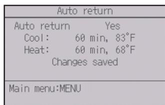
Press the [SELECT] button to save the settings. "Cool" includes "Drying" and "Auto Cool" modes, and "Heat" includes "Auto Heat" mode.
