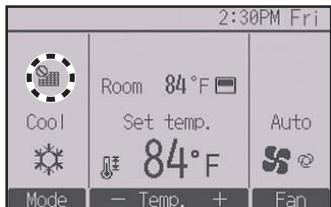
When the is displayed on the Main display in the Full mode, the system is centrally controlled and the filter sign cannot be reset.
