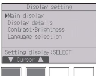
Move the cursor to “Main display” with the [F1] or [F2] button, and press the [SELECT] button.
