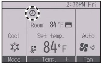
will appear on the Main display in the Full mode when the On/Off timer is enabled. The icon will not appear while the HOLD function is enabled.
