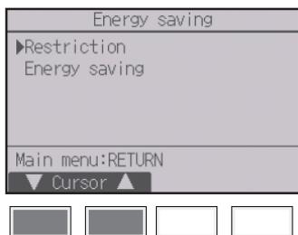
Move the cursor to “Restriction” with the [F1] or [F2] button, and press the [SELECT] button.
