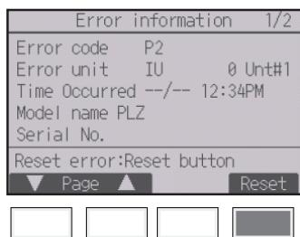
Press the **F4** button or the **ON/OFF** button to reset the error that is occurring.
