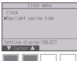
Move the cursor to "Daylight saving time" with the [F1] or [F2] button, and press the [SELECT] button.
