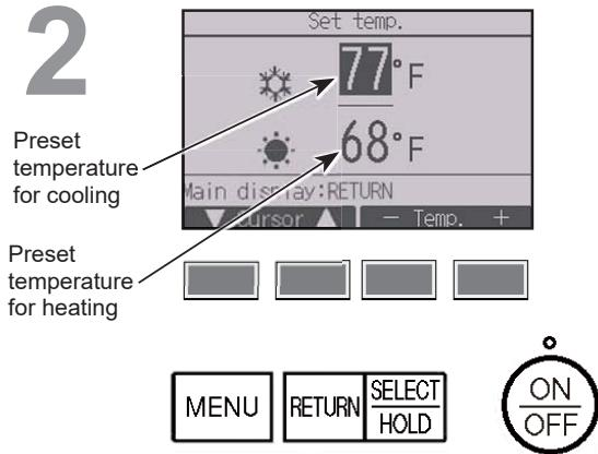
Press the [F1] or [F2] button to move the cursor to the desired temperature setting (cooling or heating).
