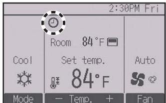
will appear on the Main display in the Full mode when the Auto-Off timer is enabled. The icon will not appear while the HOLD function is enabled.
