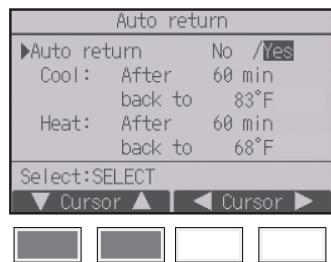
The screen to make the settings for the automatic return to the preset temperature will appear.
