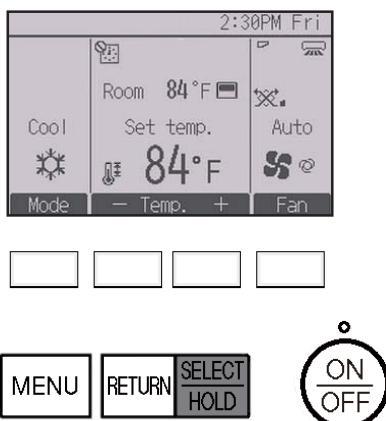
Press the **SELECT/HOLD** button to enable/disable the HOLD function.
