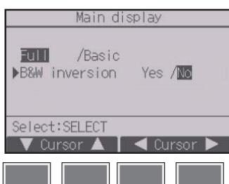
Select “B&W inversion” with the [F1] or [F2] button, and select the display mode “Yes” or “No” with the [F3] or [F4] button, and press the [SELECT] button. (The factory setting is “No.”)
