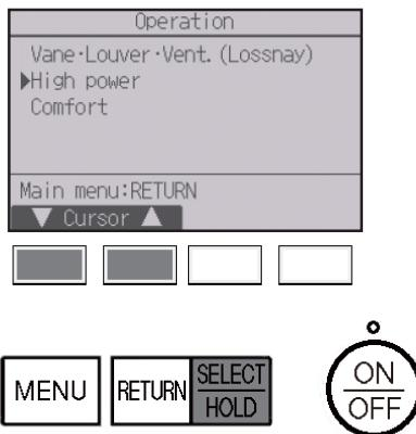
Select “High power” from the Operation menu during Cooling, Heating, or Auto operation, and press the [SELECT] button.
