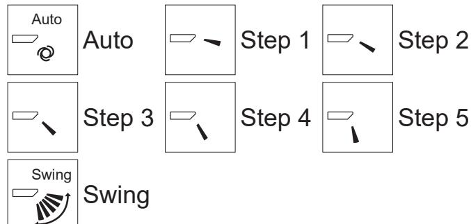
Select "Swing" to move the vanes up and down automatically.
