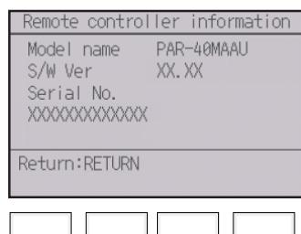
The model name, software version, and serial number of the remote controller in use can be checked.
