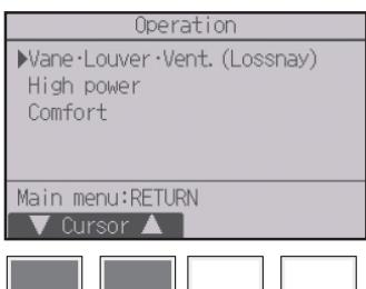
Select “Vane•Louver•Vent. (Lossnay)” from the Operation menu, and press the **SELECT** button.
