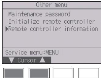
Move the cursor to “Remote controller information” with the [F1] or [F2] button, and press the [SELECT] button.
