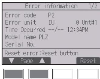
Error code, error unit, refrigerant address, unit model name, date and time on which an error occurred, and serial number will appear.
