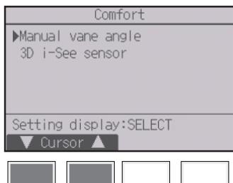
Select “Manual vane angle” with the [F1] or [F2] button, and press the [SELECT] button.
