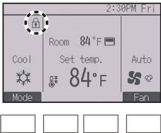
will appear on the Main display in the Full mode when the operation lock function setting is enabled.
