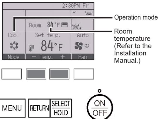
Press the [F2] button to decrease the preset temperature, and press the [F3] button to increase.
