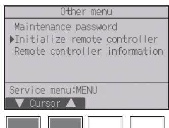
Move the cursor to "Initialize remote controller" with the **F1** or **F2** button, and press the **SELECT** button.
